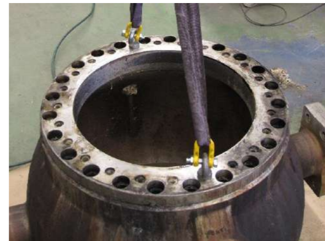
33. Attach two eye bolts to the top flange. Attach round slings and attach these to a lifting device. Start lifting to remove the clamp ring. If it is stuck, gentle heating may be applied. Do not use blunt force to remove the clamp ring as this may damage the clamp/seat ring.
