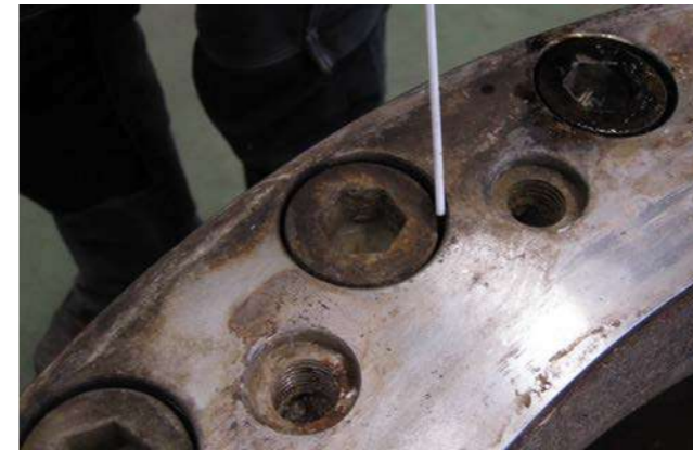
33. Attach two eye bolts to the top flange. Attach round slings and attach these to a lifting device. Start lifting to remove the clamp ring. If it is stuck, gentle heating may be applied. Do not use blunt force to remove the clamp ring as this may damage the clamp/seat ring.
