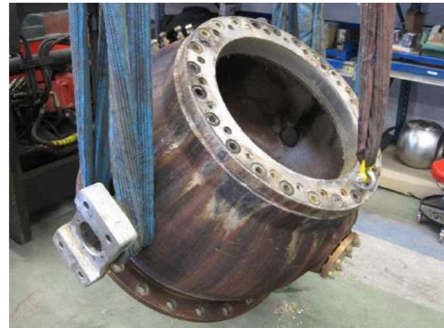
29. Hang a sling around each stem of the valve body, preferably using a crane or a forklift for a controlled simultaneous lift. Slowly lift the ProCap some 30 cm for the floor.
