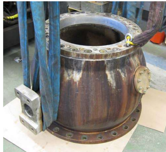
30. Attach an eye bolt to the top flange on the opposite side of the way the valve is to be turned. Attach a round sling and attach this to a lifting device.
