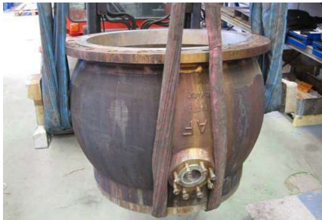
31. In a controlled manner, start to raise the upper flange thus turning the valve. Control the forklift levels upward/downwards for a controlled rotation. When the valve is fully turned, lower it onto a protected and clean surface.
