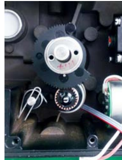
Potentiometer and cogwheel for 90° rotation
