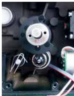
Potentiometer and cogwheel for 90° rotation
